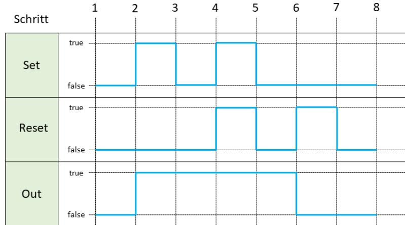
The value in the Out slot is saved in each case.
