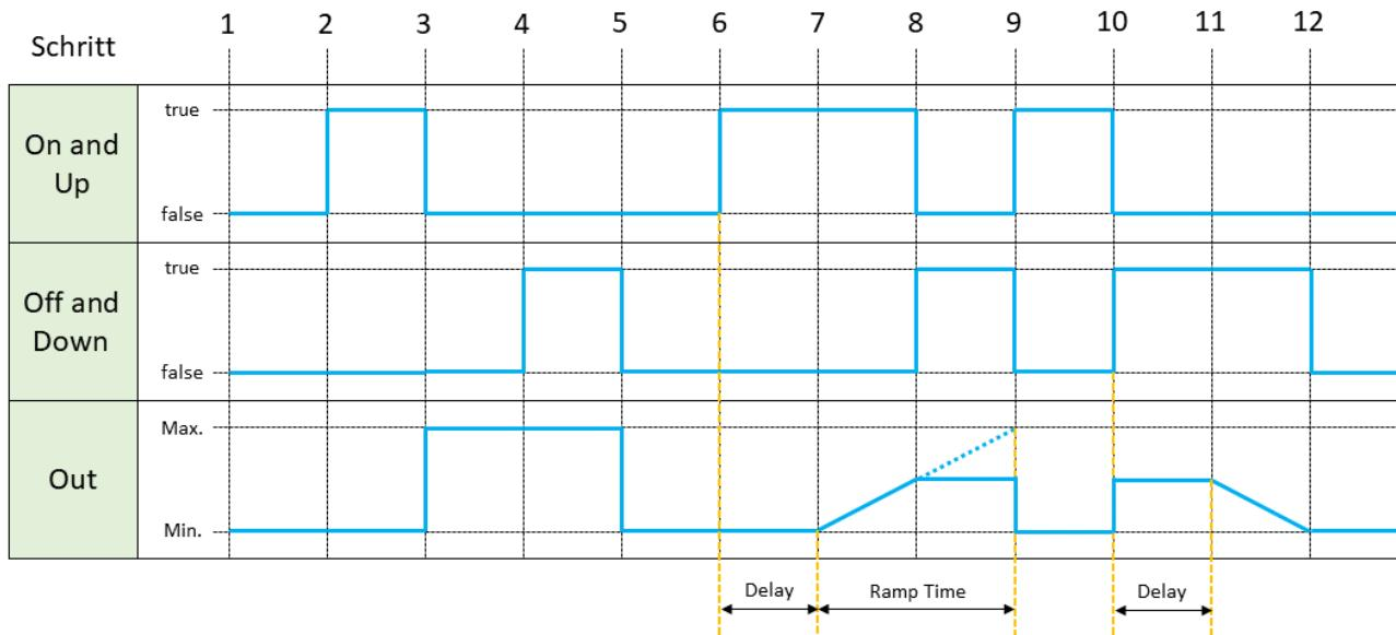
Watch out: Recognising a digital input under 300ms is difficult with Niagara, as all inputs are read in at different speeds via bus protocols. For this reason, a certain amount of caution is required when evaluating the function of the dimmer.
