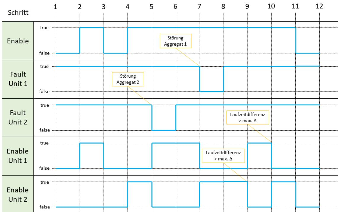
If a running genset has a fault, the second genset takes over, regardless of its running time. If a non-running genset has a fault, the runtime switchover is not carried out, even if the conditions for this would have been met. If both gensets have a fault, the Total Failure output is set to true.
