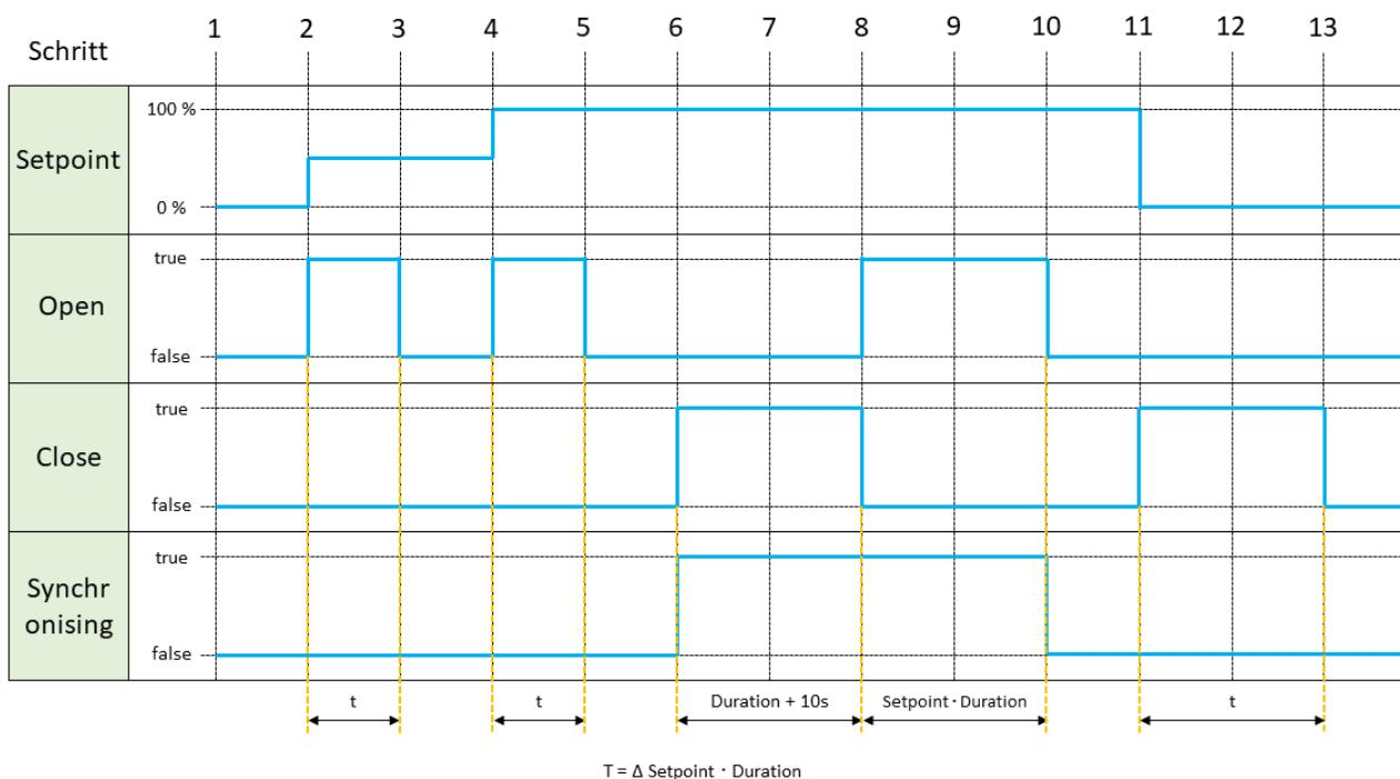
If synchronisation is switched on, the drive is fully closed during the synchronisation interval (+10s safety) and then opened again according to the setpoint. This is used to compensate for the inaccuracy that accumulates over time.
